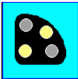
Signal: “Careful shunting allowed” (signal 44)
