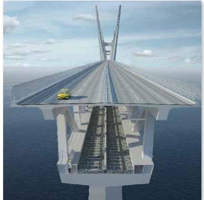
Figure 13: The Fehmarn Belt link can be designed as a two-level composite bridge in steel and concrete. Trains will run on the lower deck with cars on the upper deck. Illustration: Fehmarn Link A/S.
