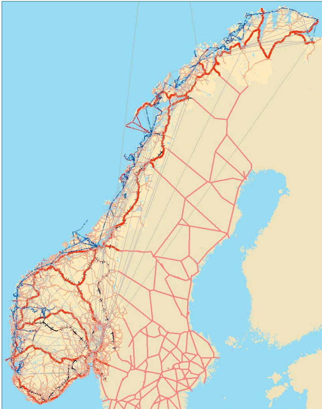
Figure 3.5. The NTM6 long distance travel demand model network. Roads are shown in red, railroads in black, air routes in grey and sea routes in blue.
