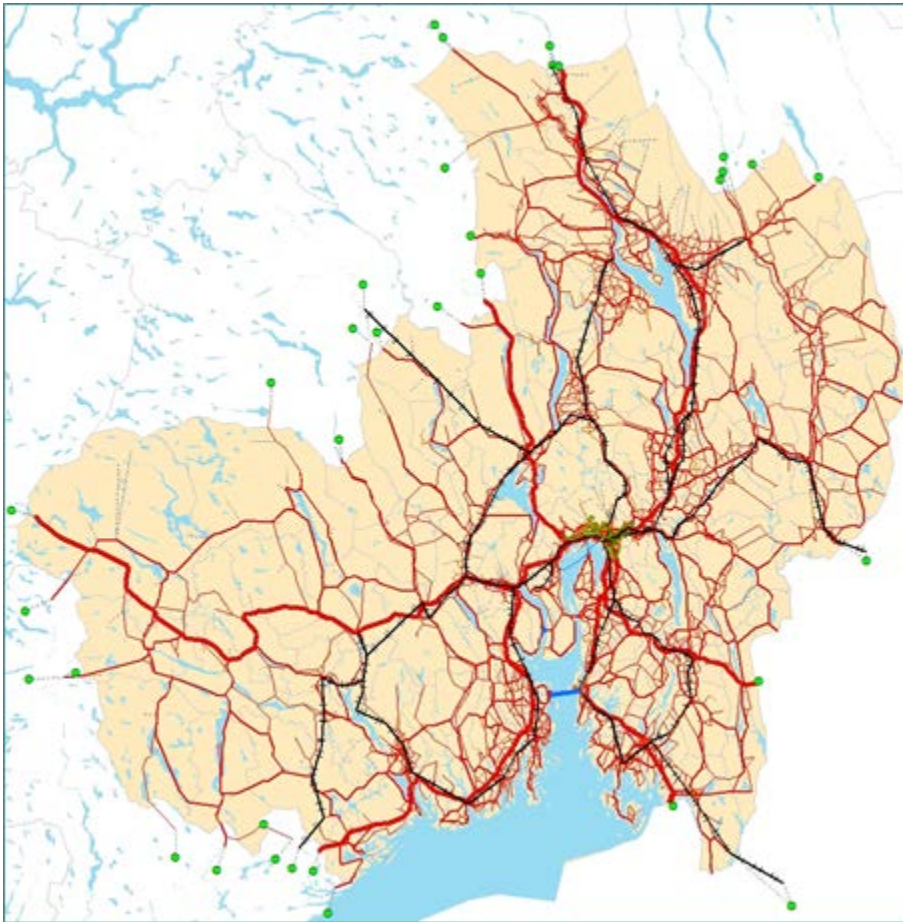
Figure 3.1. The Oslo Intercity Regional Model network for short distance trips. Roads are shown in red, railroads in black and sea routes in blue.
