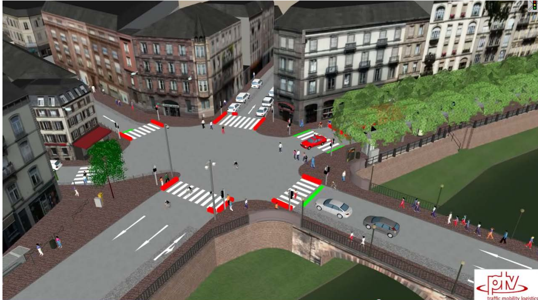
Figure 18: Vissim/Viswalk simulation of traffic, bicycles and pedestrians around Pont Kuss in Strasbourg – involving both formal and informal crossings. Source: PTV ( https://www.youtube.com/watch?v=YzPYnjHe0VU ).
