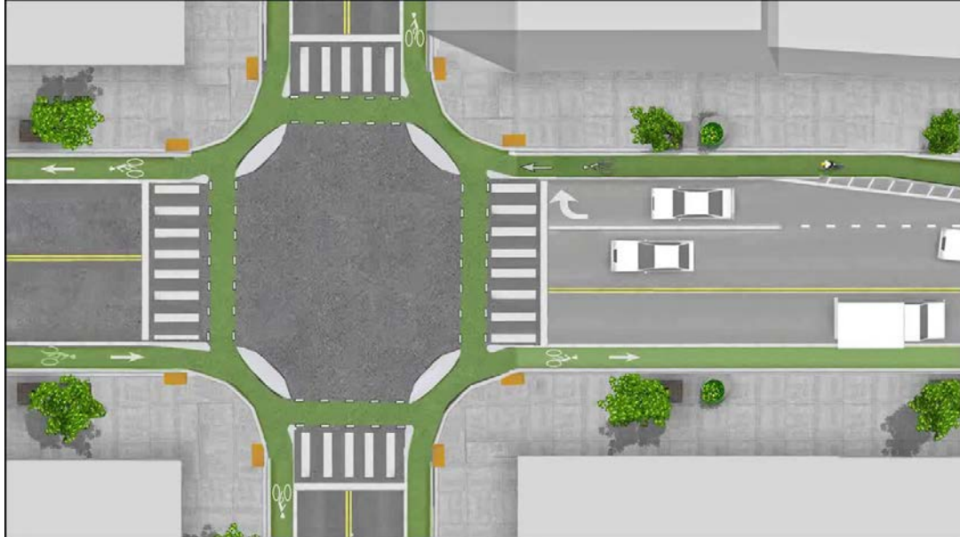
Figure 6: Illustration of common (though not only) Dutch junction design, incorporating ‘protected’ cycle lanes which allow for two-stage left turns, increase the separation between bicycles and vehicles, and create clear sightlines for points of conflict between bicycles and vehicles. Source: Mark Wagenbuur ( https://bicycledutch.wordpress.com/ ).
