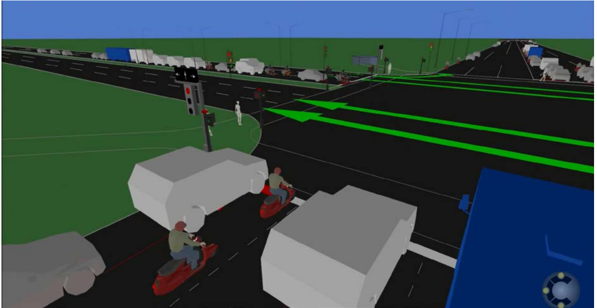
Figure 22: Example of lane sharing based on lanes being defined in Commuter as spaces available for vehicles, allowing for width-based judgements. Source: Azglient Ltd ( https://www.youtube.com/watch?v=SghIKeKoNF-A&index=12&list=PL51-5Lg_rmm2jUeljrjfuB7G.AhSxe39uDI , accessed 30.11.2014).
