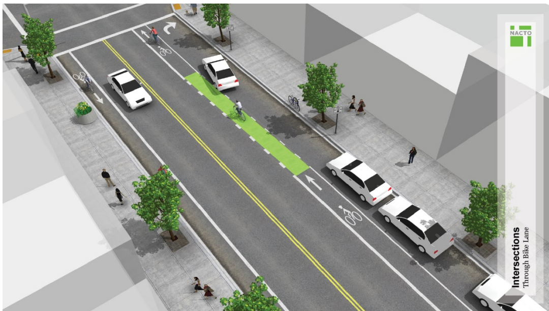
Figure 5: Revised through-bike-lane design advice, NACTO Urban Bikeway Design Guide, Second Edition . Source: NACTO Urban Bikeway Design Guide, Second Edition .
