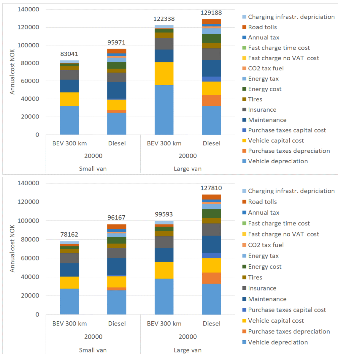
Figure 9.17: Annual costs for small and large electric and diesel LCVs in 2019 (top) and 2025 (bottom). 20,000 km/year. BEV = Electric vehicle. NOK. Source: Own calculations with TØI-TCO.
