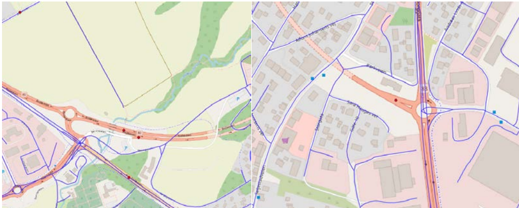
Figure 5.3: Two illustrations of mismatches between the road network and the actual location of the road.
