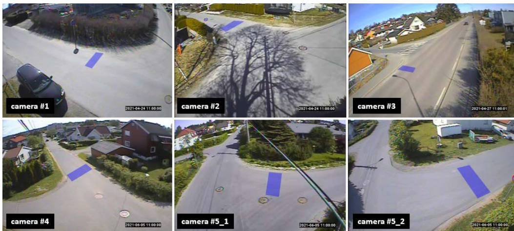
Figure 2.5: Shapes and positions of presence detectors in RUBA.
