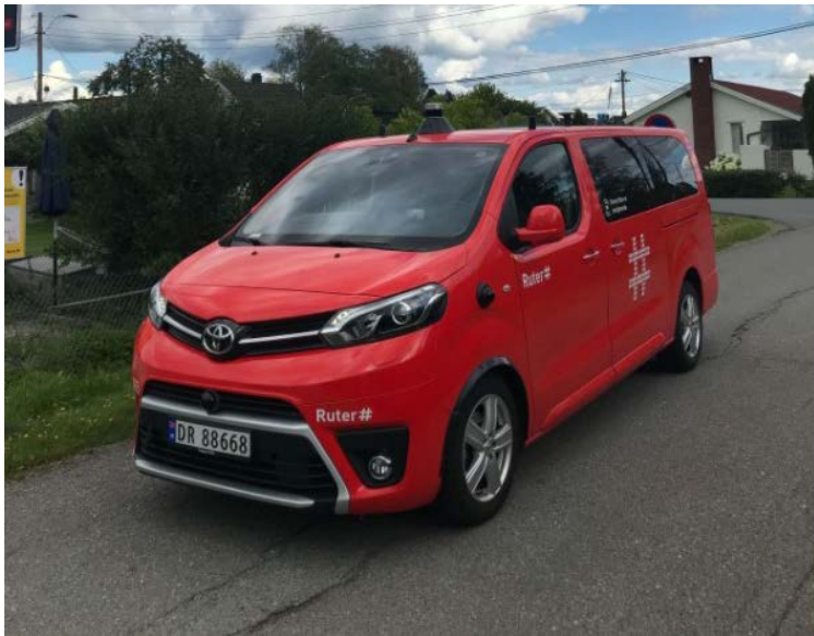
Figure 1.2: The retrofitted automated Toyota Proace van (photo: TØI).
