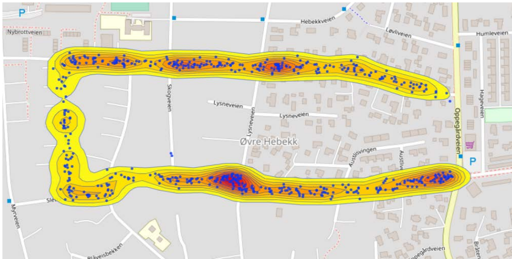
Figure 2.2: Heat map showing the locations where the shuttle stopped for a pedestrian (period 22/4 – 7/5/2021, source: Holo).
