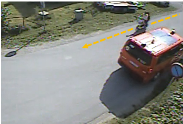
Figure 3.4: The shuttle (in automated mode) stops because of a moped riding in the opposite direction ( clip #4 ).
