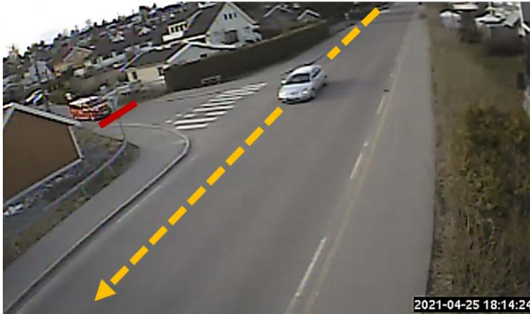
Figure 3.18: The shuttle stops too early/unnecessary when giving way to passing car. Position of shuttle and car when the shuttle stops ( clip #24 ).
