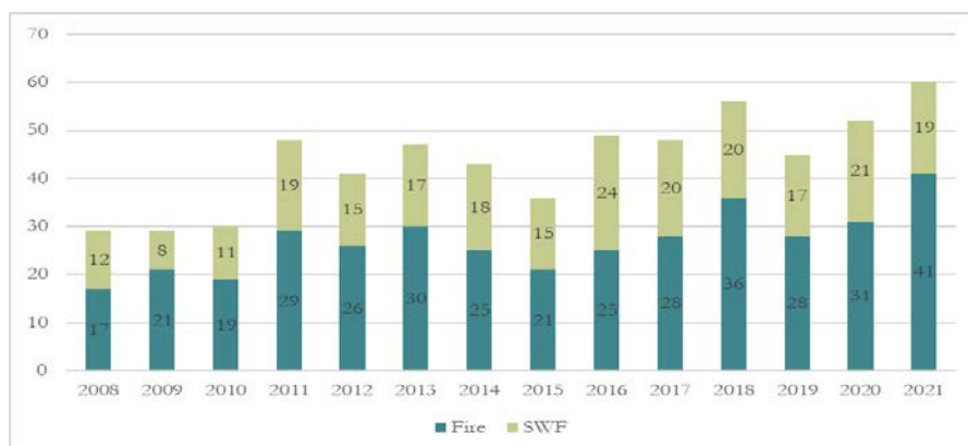
Figure S.1: Fires and SWFs in Norwegian road tunnels in the period 2008-2021 (N=613).
